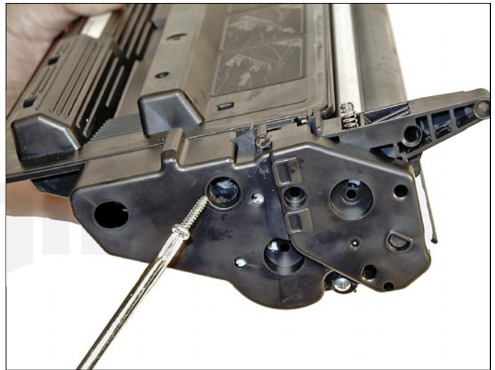
30. Install the end cap. Hold it in place with the small self-tapping screw used earlier.
