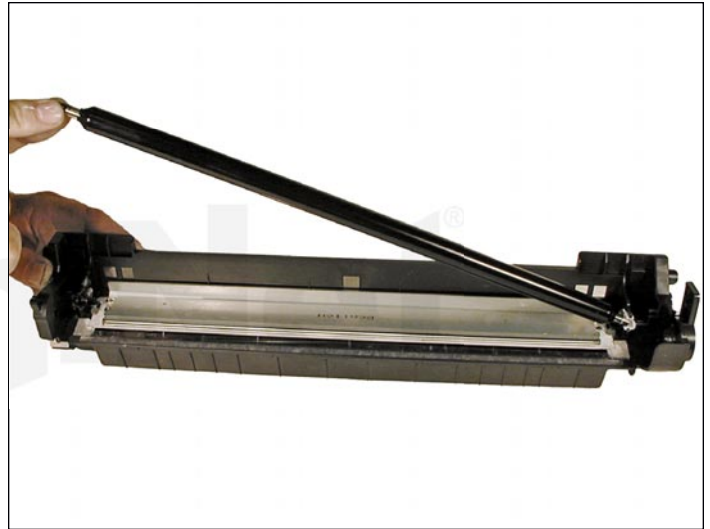
8. Remove the primary charge roller (PCR), by prying it out of the clips on either end. Clean the PCR with your preferred cleaner and place the aside.
